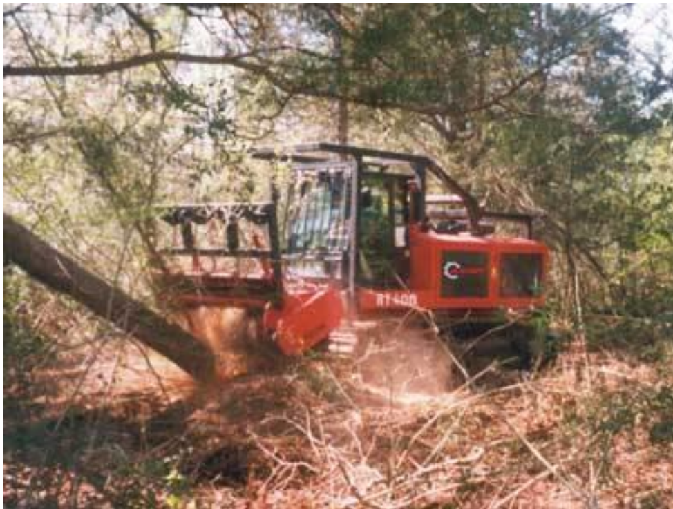
Slika 9: Primer mulčerja RT400. (Vir: Interno gradivo SCT, 2005)
