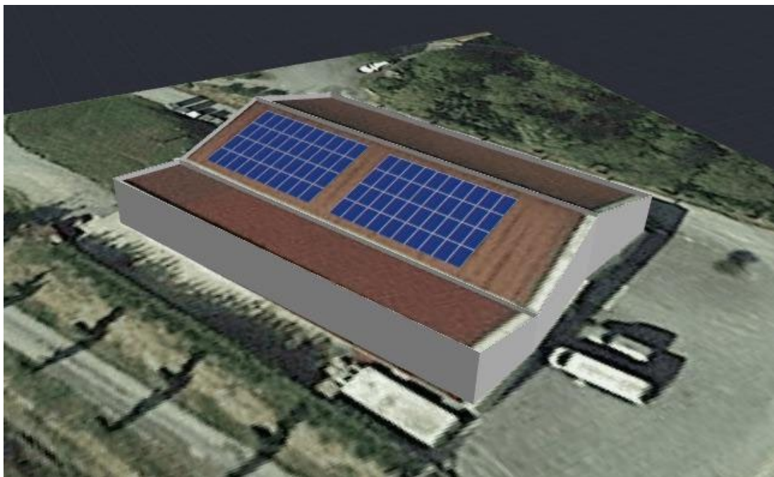
Slika 6: Izris PV modulov (Vir: SolarEdge designer, 2024)
