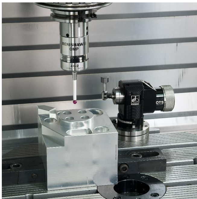
Slika 29: Merilna sonda in naprava za kalibriranje orodja (Vir: https://www.renishaw.com/en/ots-3d-touch-trigger-tool-setter--6783 )
