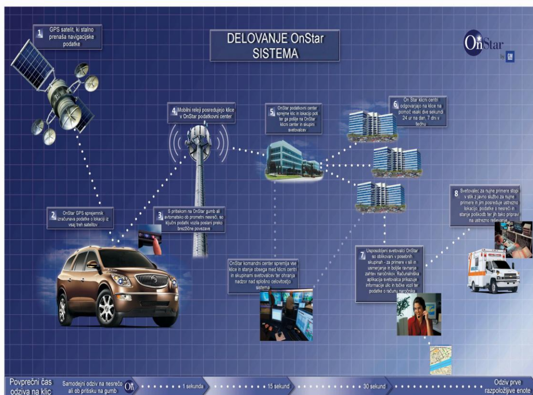
Slika 7: Prikaz delovanja OnStar sistema (vir: http://qmauthority.com/blog/wp-content/uploads/2011/06/How-OnStar-Works-small1.jpg – prevod: lasten )
