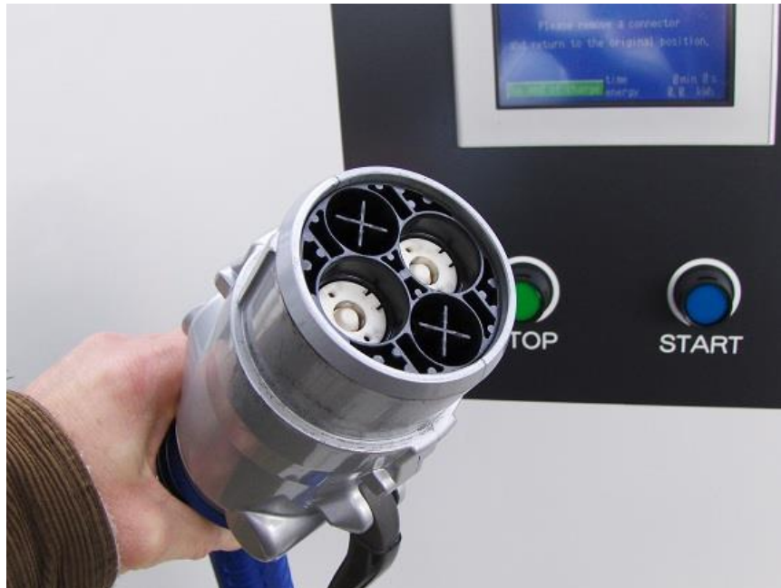
Slika 7: Tip CHAdeMO (Vir: Green Transportation.si, 2019)
