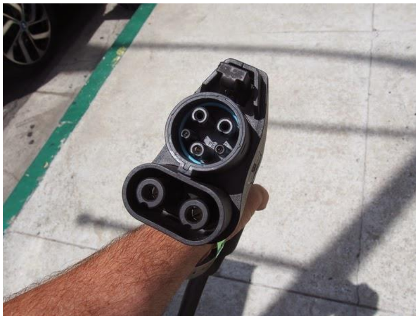
Slika 8: Tip Combo 2 (Vir: Green Transportation.si, 2019)
