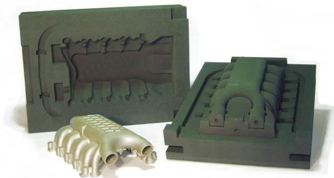
Slika 6: Livarska forma (interno gradivo Chemets d.o.o.)
