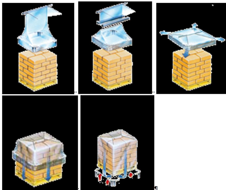
Slika 3: Faze pri pakiranju nove tovarne enote z raztegljivim polivinilom (Vir: Baumer sistem za ovijanje http://www.beumer.com/products/packaging-systems/stretch-hooding/stretch-hoodr-m/ )
