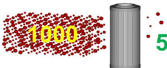
Slika 5: Primer 1: \beta_{6(c)} = 200 (Vir: Hyprofiltration 2020)
