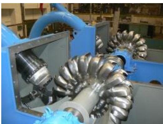
Slika 3: Peltonova turbina (Vir: Hočevar in Dular, 2015, str. 19)
