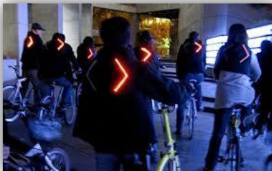
Slika 19: Smerniki za nakazovanje smeri levo in desno na hrbtnem delu jopiča (Vir: https://encrypted-tbn3.gstatic.com/images?q=tbn:ANd9GcTzN-wTpXAcuKTC28kFylg_cvYymZ1DykWwrEf2vha4QxJiy7Rf )
